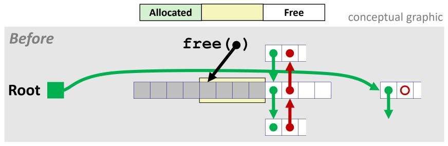
Splice out adjacent successor block, coalesce both memory blocks, and insert the new block at the root of the list
